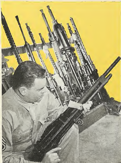
Firepower of enemy guns is tested at Wright Field. Weapons shown here include (left to right) Italian Breda 8 mm flexible machine gun (held by sergeant), Breda 12.7 mm (flexible), Breda 7.7 mm (flexible), German 7.9 mm (flexible), another Breda 7.7 mm, German Oerlikon 20 mm fixed cannon, Oerlikon 20 mm flexible cannon, two German MG-17 7.9 mm fixed machine guns, Jap 7.9 flexible machine gun and an AAF .50 caliber machine gun.
